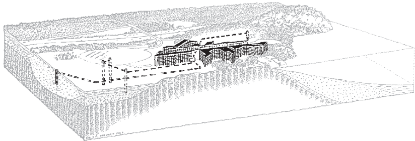
Figure 4: The Frösundavik Aquifer with three cold wells in the center and the warm wells in the surrounding areas
