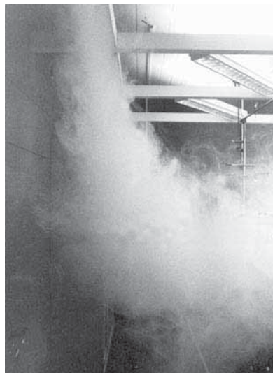
Figure 12: The fresh air flows above the vortex falling from the ceiling
