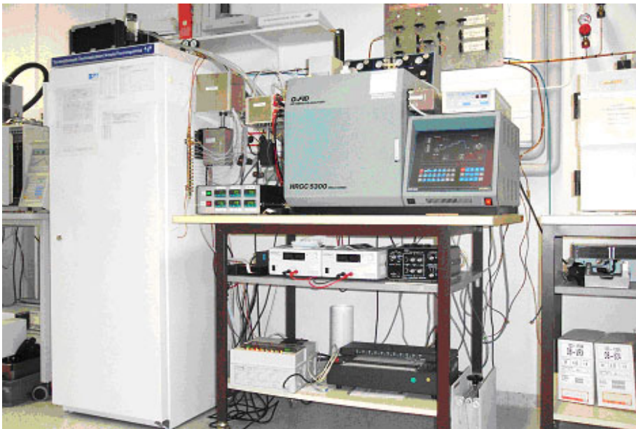
Figure 46: Ultra permeation measurement unit.
