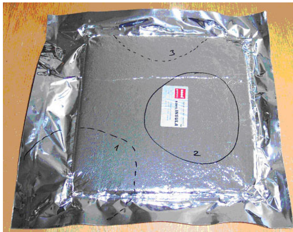
Figure 44: Sample preparation for the permeability measurements.
