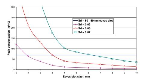
Figure 5 . peak accumulated condensate as a function of eaves gap and underlay resistance.
