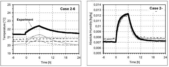
Measured values and simulation results (ventilation rate: 0.64 ach, ambient temperature 20.5°, ambient relative humidity 51%, all walls non-buffering)
