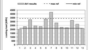
Figure 1. A comparison of annual net energy demand for heating and cooling for heavyweight structure building between various models in Common Exercise 0. The dotted and the full lines give the simulated maximum and minimum values from Annex 21.
