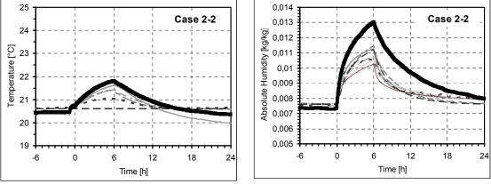
Measured values and simulation results (ventilation rate: 0.62 ach, ambient temperature 20.6°, ambient relative humidity 51%, floor covered with gypsum board)
