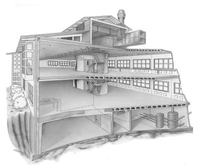
Figure 5.6 - Typical built up of the ventilated hollow concrete core slab system - TermoDeck®.
