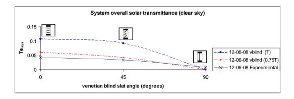
Figure 4B.2 - System overall solar transmittance for different slat angles under CSC.
