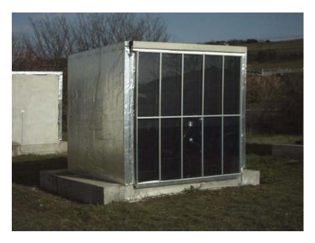
Figure 7.6 – Example of an experimental passive solar wall making use of PCM (Experimental test facility at Università Politecnica delle Marche - Italy).
