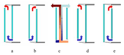
Figure 4.3 - AIF flow path: a) EA; b) SA; c) RAF; d) OAC; e) IAC [State-of-the-Art Report Annex 44 (2005)].
