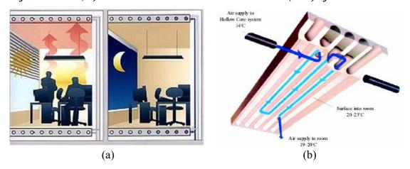
Figure 5.4 - Examples of TMA - CA systems. a) Principle of the Thermo Active Building System - TABS (www.velta.de/ October 2006); b) Principle of the TermoDeck® system.
