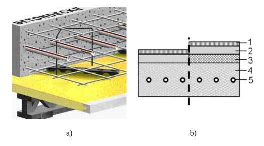
Figure 5.7 - a) Cross-section of the on-site constructed system (www.uponor.de/ August 2008); b) TABS with and without acoustic insulation, 1=floor surface covering, 2=screed, 3=acoustic insulation, 4=building structure and 5= plastic pipes [Babiak et al. (2007a)].
