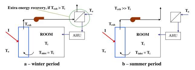
Figure 4.31 – Operating strategies of the ventilated façade and integration with the HVAC system.
