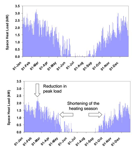
Figure 8.8 – Heating loads assessed for the Balerno building without the DI (top), heating loads assessed for the Balerno building with the DI element installed in the roofs (Top).
