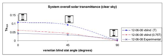
Figure 4.14 - System overall solar transmittance for different slat angles under CSC.
