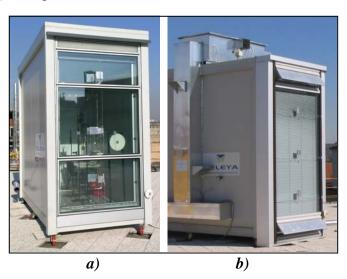
Figure 4C.1 – pictures of: a) Climate façade, b) Hybvent DSF.
