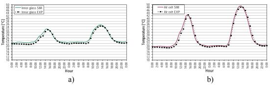
Figure 4.10 – Simulated (continuous lines) and measured (symbols) glass (a) and air (b) temperatures, roller screen configuration.
