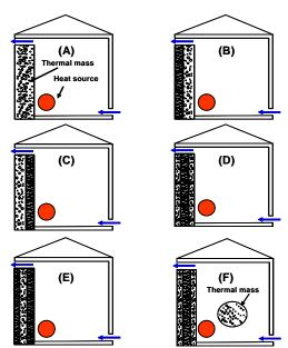
Figure 5.2 - Illustration of six simple building models with different relative location of the thermal mass to the insulation and the existence of internal thermal mass [Li and Xu (2006)].
