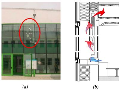
Figure 4.30 – (a) The monitored climate façade at the Environment Park, in Turin, Italy –(b) Scheme of the working principle of the façade at the Environment Park, in Turin, Italy.
