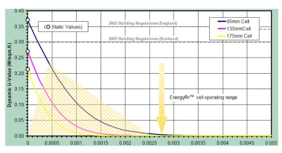
Figure 8.6 - Variation of dynamic U-value of walls incorporating Energyflo  $^{TM}$  cells with the variation of inward air flow rate through the cells.
