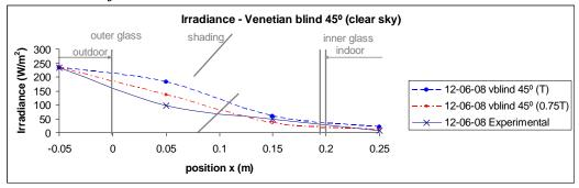
Figure 4.13 - Irradiance for different slat angles under Clear Sky Conditions. Experimental and numerical data (numerical results obtained for T, the glass manufacturer transmittance, and 0.75T).
