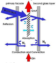
Figure 4.1 - DSF/AIF working principles.
