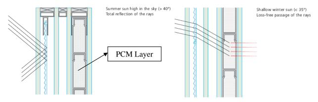
Figure 7.7 – Working principles of a passive solar wall (GLASSX type) making use of PCM.
