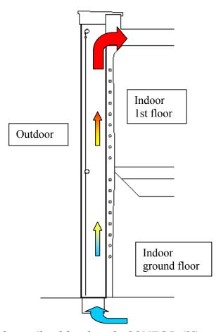
Figure 4.36 – Scheme of the ventilated façade at the SOMEC Building.
