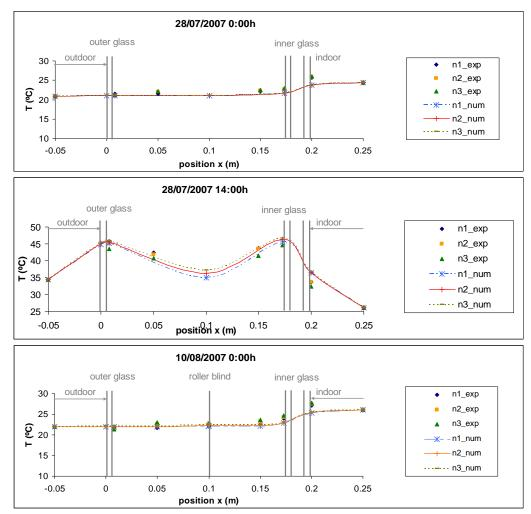
Figure 4.15 - Comparison between experimental (LNEC test cell – section 4.3.4.2) and numerical results.
