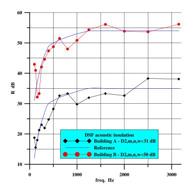
Figure 4.23 – Example of measured acoustic insulation,  $D_{n,w}$ , in two different buildings with double skin façades.
