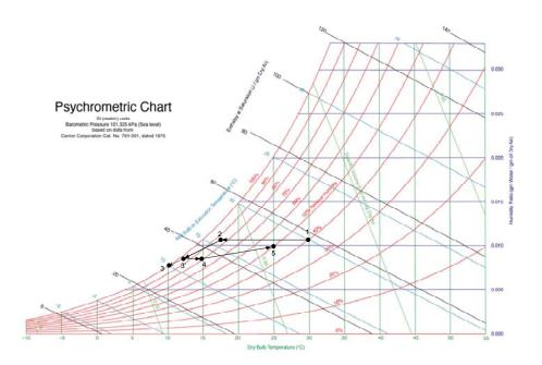
Figure 6.4 - The Psychrometric chart presentation of air cooling processes in an ETAHE, 1: outdoor air condition; 2: transition condition (condensation starts); 3: duct surface condition; 3': ETAHE outlet air condition; 4: room supply air condition; 5: room air condition.
