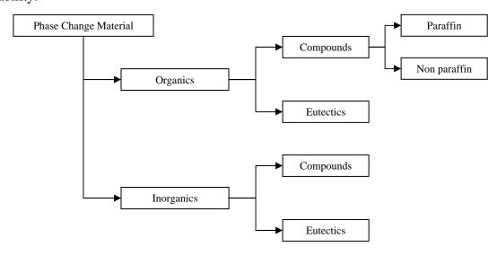
Figure 7.2 – Different typologies of Phase Change Materials (PCM).
