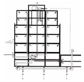
Figure 6.9 - Schematic of Schwerzenbacherhof building ventilation system [Hollmuller (200)]).
