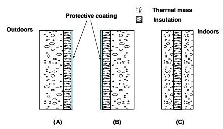
Figure 5.22 - The placement of mass relative to the insulation can be critical in regard to time lag as well as have other implications. (A) Mass on outside – interior insulation (B) Mass on inside (C) Mass sandwich [Adapted and modified from Lechner, (2001)].
