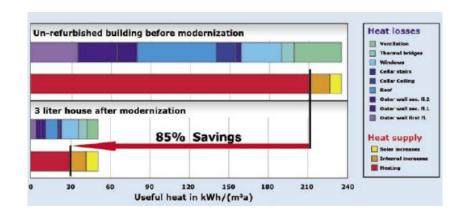
Figure 7.17 - "3-Litre" house -Energy certificate before/after the energy retrofit.
