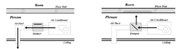
Figure 5.29 - Control of damper (left: working hours, right: thermal storage hours).
