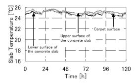
Figure 5.33 - Vertical distribution of floor slab temperature at measuring point number 3 (left) and number 4 (right).
