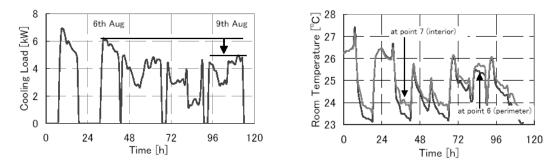
Figure 5.28 - Cooling load (left) and room air temperature (right) for measuring points number 6 and 7 of the examined room in KANDEN building.
