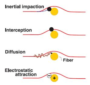
Figure 8.2 - Four primary particle collection mechanisms of particle capture.
