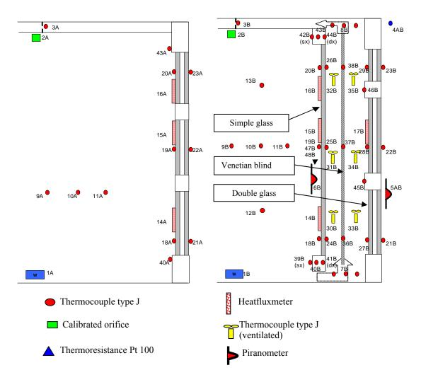
Figure 4.17 – Scheme of the sensors for the reference and the test façade (for this test cell, the set-up may vary, depending on the type of component under test).
