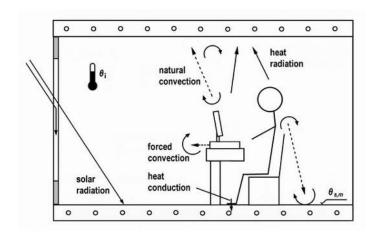
Figure 5.20 - Thermal balance model of a room equipped with radiant heating/cooling [Koschenz and Lehmann (2000)].
