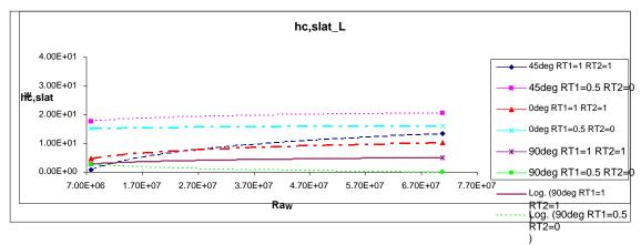
Figure 41.1 -. Calculated hcw for different slat angles and temperature conditions.
