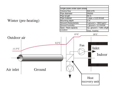
Figure 6.6 - ETAHE with heat recovery during the winter operation [Fink et al. (2002)].
