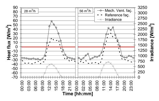
Figure 4C.4 – "Long wave" heat fluxes entering the climate and the reference façade, winter conditions.
