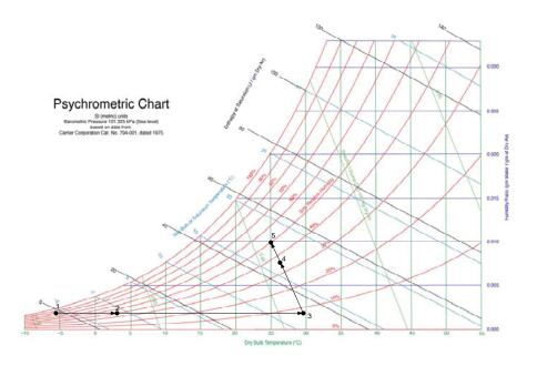
Figure 6.5 - The Psychrometric chart presentation of heating processes of ETAH - 1: outdoor air condition; 2: ETAHE outlet air condition; 3: air condition after secondary heating; 4: mixing air condition; 5: return duct air condition.
