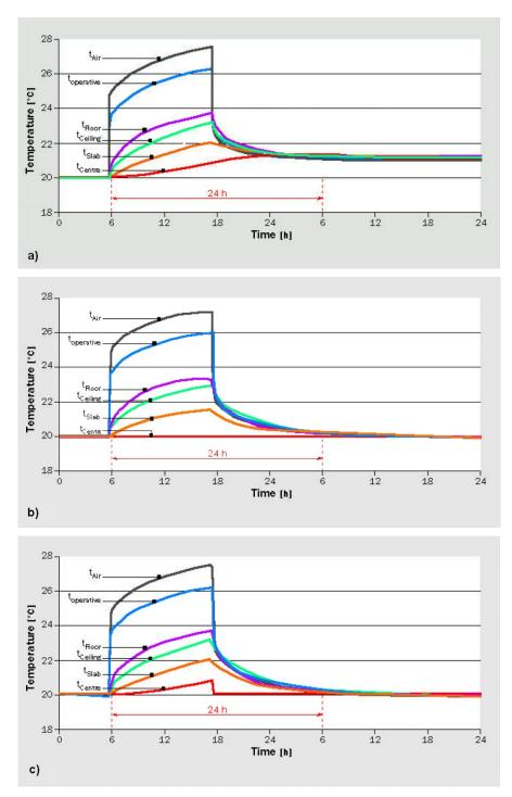
Figure 5.23 - Core thermal mass activation: calculated air, operative, floor, ceiling, average slab and slab core temperatures for a space with a constant internal load of 90  $W/m^2$  from persons, light, solar radiation etc. [Meierhans and Olesen (1999)].
