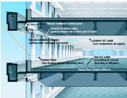
Figure 5.27 - Existing application of ACSuBTS - KANDEN Building of Kansai Electric Power Company, Inc. (KEPCO) in Osaka.
