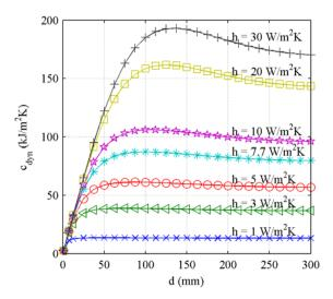
Figure 5.12 - Diurnal heat storage capacity,  $c_{dyn}$  of a concrete slab depending on the thickness, d for different heat transfer coefficients, h.
