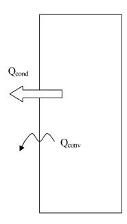
Figure 8.2A - Heat flux in the exterior surface of DI.
