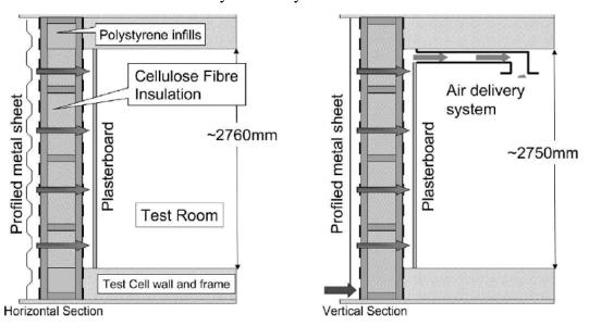
Figure 8.3 - Prototype design of dynamic insulation wall [Baker, (2003)]
