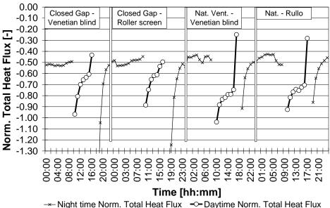
Figure 4C.5 – Normalized total heat flux, hybrid ventilated façade, winter conditions.
