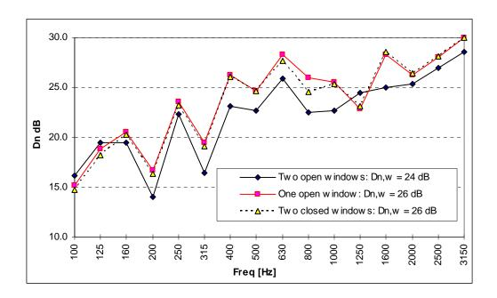
Figure 4F.1– Measured airborne acoustic insulation,  $D_{n,w}$ , from office to office, in building B, proved to be poor mainly due to the sound transmission by the ceiling and interior doors. The small difference between one and two closed windows reflects the individual window good insulation.
