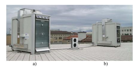
Figure 4.16 – pictures of: a) Façade under test (in this case a hybrid ventilated façade), b) Reference façade.
