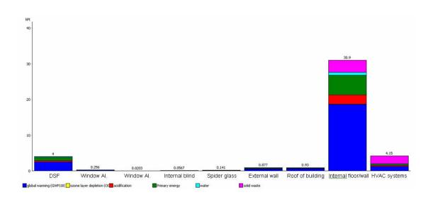
Figure 4H.3 – Environmental load in construction phase of an office building with DSF.
