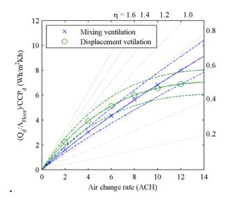
Figure 5.14 - Heat discharged during night-time ventilation per unit floor area and daily CCP depending on the air change rate; based on experimental results for mixing and displacement ventilation (including range of uncertainty) and lines of constant efficiency  $\eta$ ; room height H = 2.93 m.
