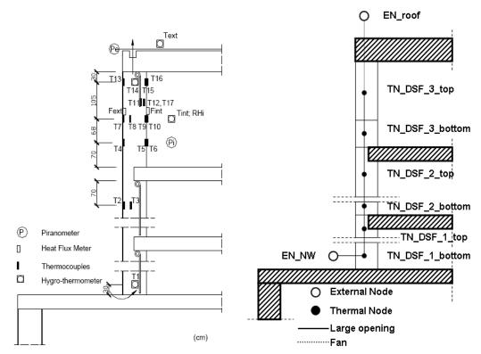
Figure 4.5 - Sketch of the measured façade and numerical model.
