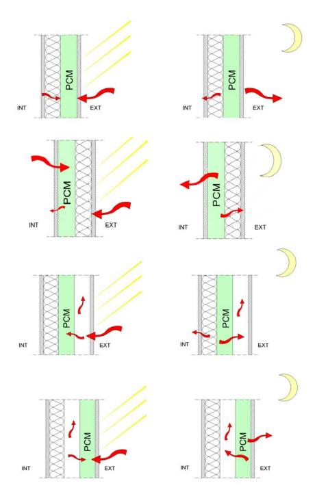
Figure 7.3 – Scheme of the possible working principles of walls making use of PCM.
