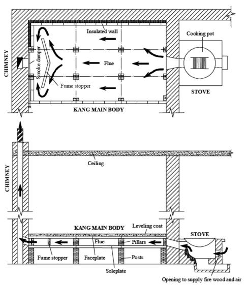
Figure 5.38 - A complete illustration of elevated kang domestic heating system including the chimney, the kang and the stove.
