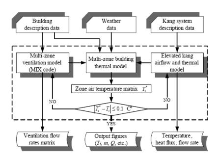
Figure 5.39 - The implementation procedure of the HIEK model [Li et al. (2007)].
