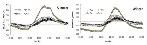
Figure 4.48 - AIF(NV-OAC), Total thermal load includes heat transmission through interior pane and solar radiation passed through interior pane(positive values show gains). AIF is ventilated naturally.
