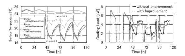
Figure 5.37 - Calculated lower surface temperature of the slab (left) and cooling load (right) when air circulation is improved.
