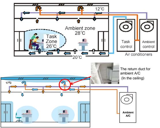
Figure 5.28 - Air conditioning system utilizing building thermal storage – operation principle.
