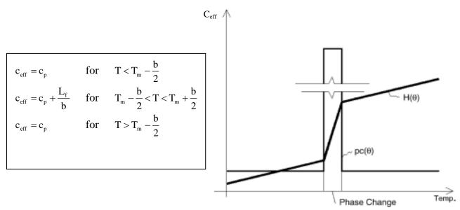
Figure 7.12 – Effective heat capacity of PCM vs. Temperature (example of non continuum function).
