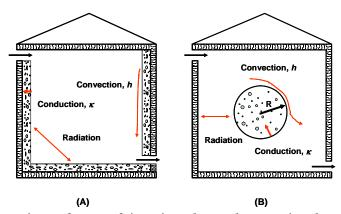
Figure 5.21 - (A) Illustration of use of interior thermal mass in the walls, floor; and (B) Illustration of the heat transfer process of a thermal mass sphere in a room. [Li and Xu (2006)].
