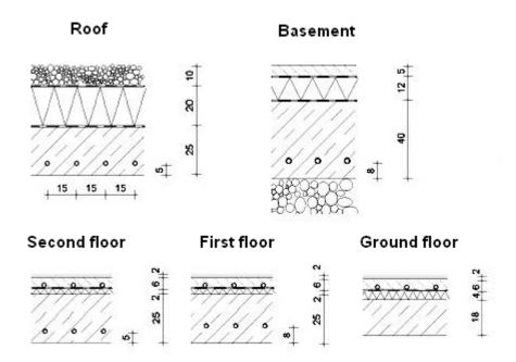
Figure 5.41 - Different positions of pipes as used in the ZUB in building Kassel, Germany [De Carli et al. (2003)].
