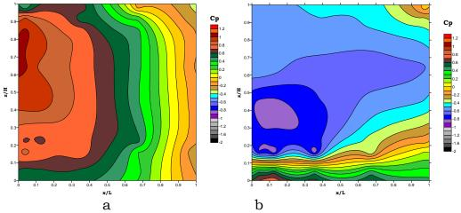
Figure 4G.1 -  $C_p$  distribution over an "unsheltered" envelope a), and a MS-DSF b), for a 45° (corner) wind incidence.
