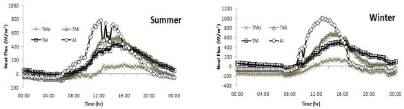
Figure 4.45 - AIF(MV-IAC), Total thermal load includes heat transmission through interior pane, solar radiation passed through interior pane and enthalpy changes of ventilation air supplied to room (positive values show gains).
