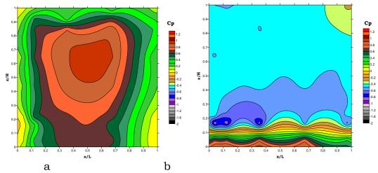
Figure 4.20 -  $C_p$  distribution over an "unsheltered" envelope a), and a MS-DSF b), for a 0° (perpendicular) wind incidence (The DSF has a multi-storey configuration, open at the bottom and top and closed on the sides. The bottom edge of the DSF is 3 m above ground level, and the cavity has a depth of 0.8 m [Marques da Silva, F. and MG. Gomes (2005)].
