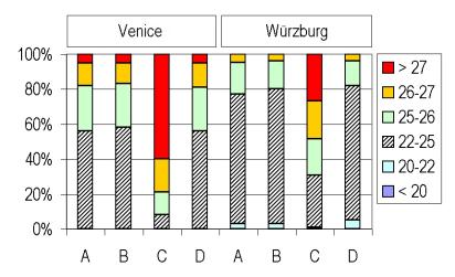
Figure 5.17 - Simulated operative temperature distribution for different water temperature control strategies: A:  $\theta_{mean} \approx f(\theta_{outdoor}, \theta_i)$ , B:  $\theta_{supply} \approx f(\theta_{outdoor}, \theta_i)$ , C:  $\theta_{mean} \approx const$  (22°C in summer, 25°C in winter), D:  $\theta_{mean} \approx f(\theta_{outdoor})$  (figure based on the data from [Olesen and Dossi (2004)]).
