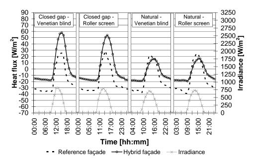
Figure 4C.3 – "Long wave" heat fluxes entering the hybrid and the reference façades, winter conditions.
