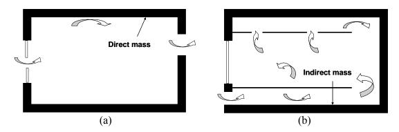
Figure 5.19 - Direct and indirect interaction thermal mass [CIBSE (2001)].
