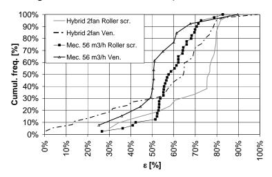
Figure 4C.9 – Dynamic insulation efficiency of the two active façades.
