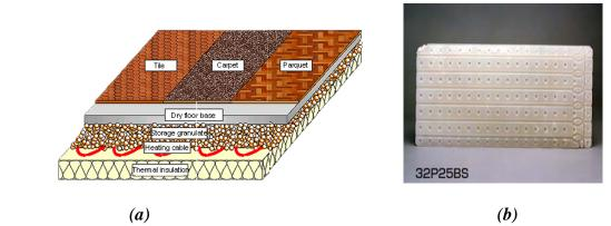
Figure 7.8 – (a) A typical configuration of a floor heating system coupled with of PCM. (b) Example of a PCM container for floor.
