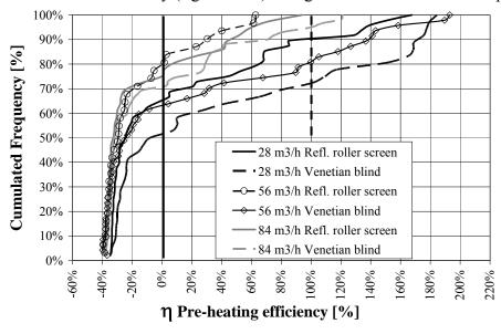
Figure 4C.8 – Pre-heating efficiency for the climate façade.
