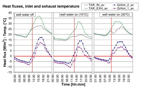
Figure 4.38 – Heat fluxes for different control strategies for the activation of the pre-cooling.
