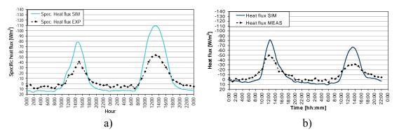
Figure 4.11 – Simulated and measured heat fluxes, roller screen (a) and venetian blind (b) configuration.
