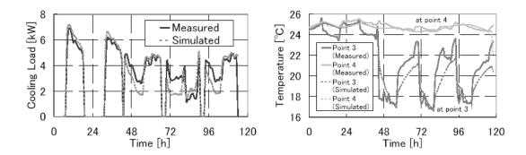
Figure 5.35 - Comparison of measured and simulated results (left: cooling load, right: lower surface temperatures of slab at points 3 and 4).
