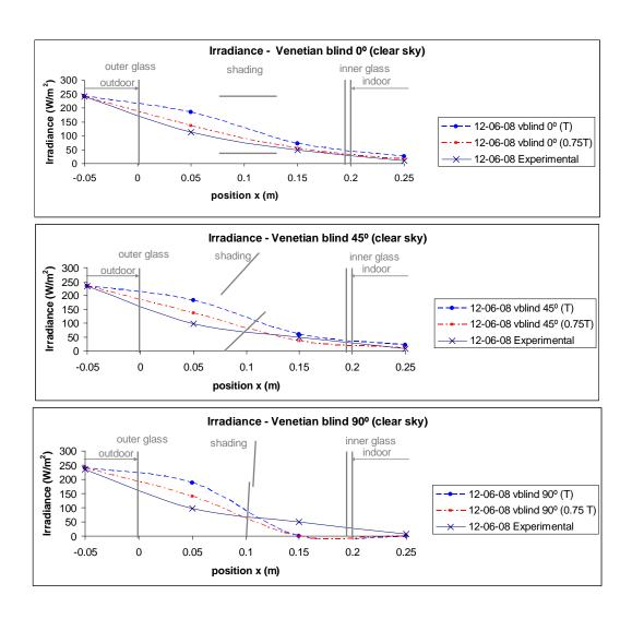
Figure 4B.1 - Irradiance for different slat angles under CSC. Experimental and numerical results for T (the glass manufacturer transmittances) and 0.75T.
