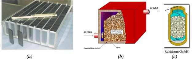
Figure 7.11 - Picture (a) and schemes (b and c) of typical storage devices based on PCM.
