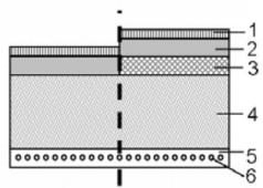
Figure 5.10 - Example of TMA - CA system: TABS with capillary micro-pipes embedded in a layer at the inner ceiling surface with and without acoustic insulation, 1=floor surface covering, 2=screed, 3=acoustic insulation, 4=building structure, 5=plastic micro-pipes and 6=plaster or gypsum [Babiak et al. (2007a)].
