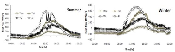
Figure 4.47 - AIF(MV-EA), Total thermal load includes heat transmission through interior pane and solar radiation passed through interior pane (positive values show gains. The amount of room air that will be exhausted through AIF was assumed to be infiltrated from surrounding warm zones of attached room).
