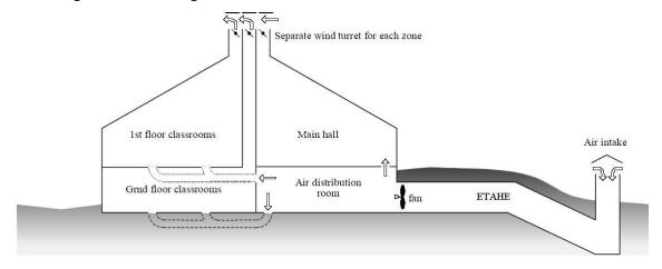
Figure 6.16 - Schematic cross section of Jaer School showing air flow paths and components' locations [Schild (2002)].
