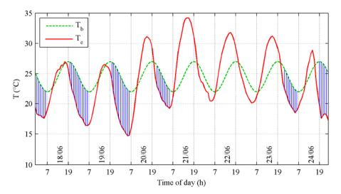
Figure 5.11- Building temperature,  $T_b$  and external air temperature,  $T_e$  during one week in summer 2003 for Zurich SMA (ANETZ data). Shaded areas illustrate graphically the climatic cooling potential, CCP.
