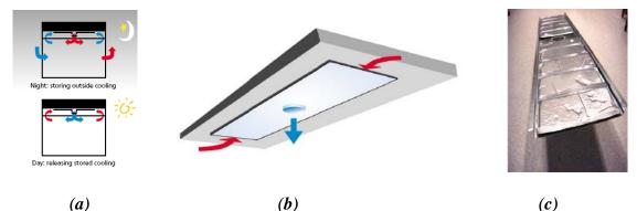
Figure 7.10 – (a) and (b) Scheme of the working principle (summer period) of a PCM based ceiling.
