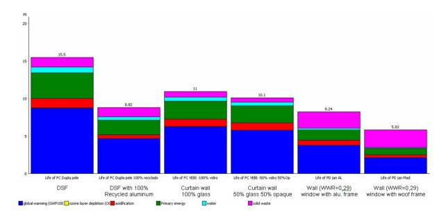
Figure 4H.1 – Environmental load of façades (table 4H.1) construction and disposal phases.
