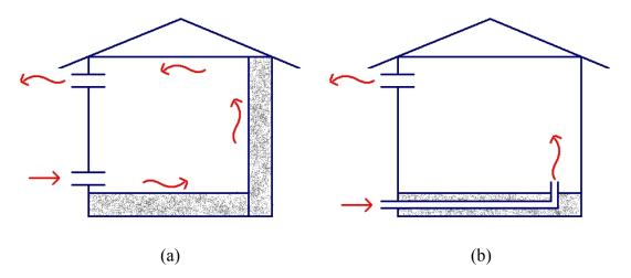
Figure 5.3 - Thermal mass activation working principles: a) SA: activation involves only the surface of the element; b) CA: activation involves whole structure (core) of the element.
