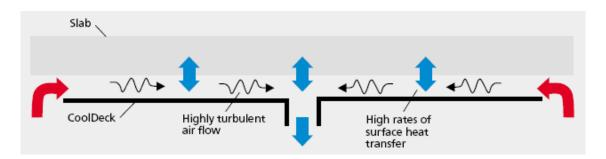
Figure 7.21 – "Stevenage Borough Council" building - Scheme of the working principle of the PCM based ceiling (Cooldeck technology).
