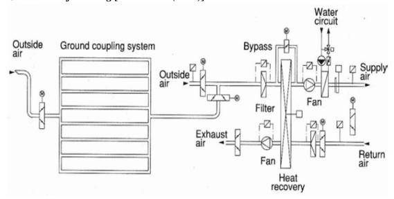
Figure 6.11 - Schwerzenbacherhof building - Ventilation system's components [Hollmuller (2002)].
