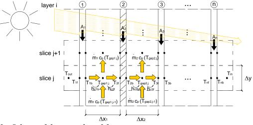
Figure 4.12 - Scheme of the network model.
