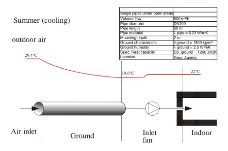
Figure 6.7 - ETAHE with heat recovery during the summer operation [Fink et al. (2002)].
