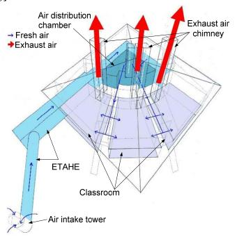
Figure 6.17 - 3D schematic of Jaer School ventilation system [Schild (2002)].
