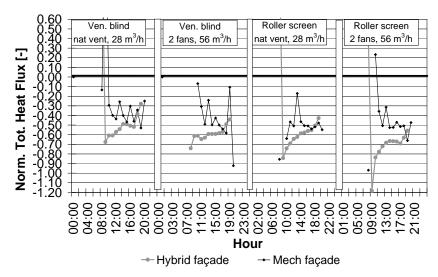
Figure 4C.10 – Normalized total heat fluxes, summer conditions.
