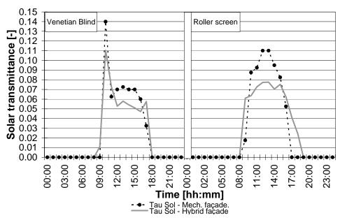
Figure 4C.7 – Solar transmittance coefficient for the monitored AIFs.
