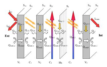
Fig. 4.8 – Heat fluxes for each horizontal zone.
