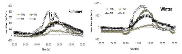
Figure 4.46 - AIF(MV-SA), Total thermal load includes heat transmission through interior pane, solar radiation passed through interior pane and enthalpy changes of ventilation air exhausted to room (positive values show gains)
