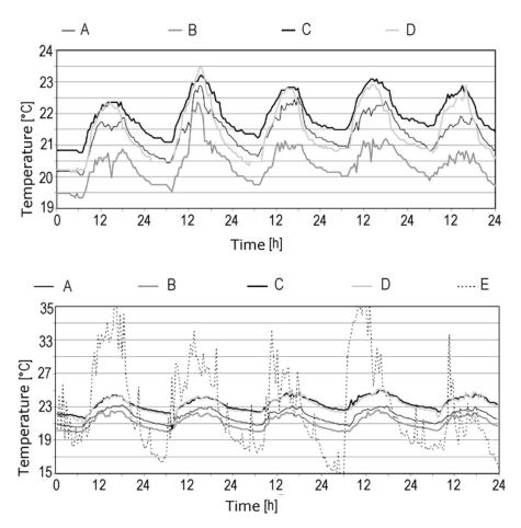
Figure 5.18 - Sample of operative temperatures measured during a working week in the heating season (top) and the summer season (bottom) in an office building equipped with active thermal mass heating/cooling system; A - 4th floor east, B - 4th floor south, C - 5th floor east, D - 5th floor west, E - outside temperature (bottom figure only) [De Carli (2002)].
