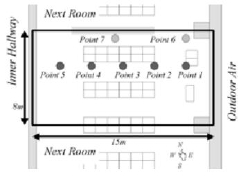
Figure 5.30 - Position of measuring points at the typical floor of the KANDEN building.
