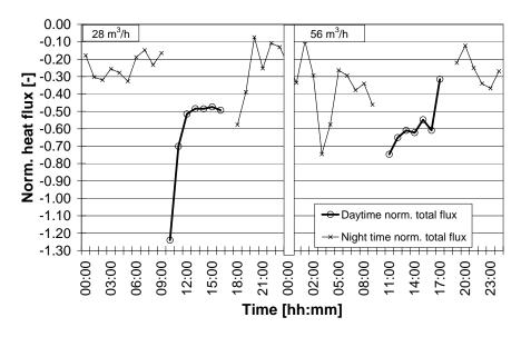
Figure 4C.6 - Normalized total heat flux, mechanical ventilated façade.
