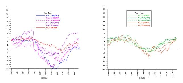
Figure 4D.7 - Temperature differences between indoor and outdoor for OAC, SA and EA.
