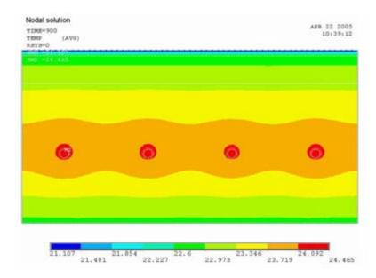
Figure 5.15 - Temperature distribution calculated by FEM software [Babiak et al. (2007b)].
