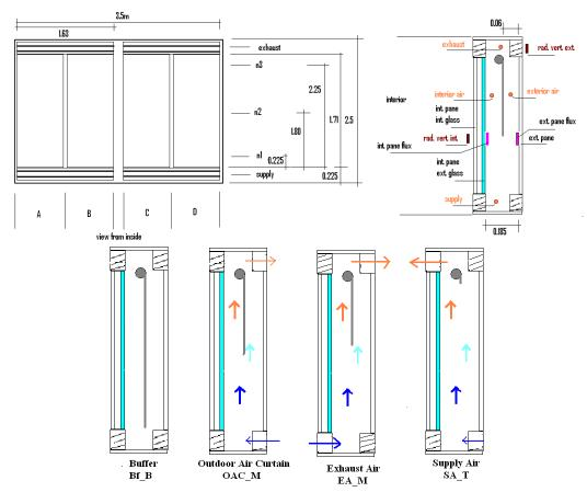
Figure 4.19 – Scheme for measuring levels and test facility sensors and the tested configurations.
