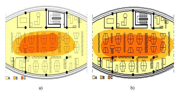
Figure 4.21 – Daylight distribution in a building with double skin façade: A – Good to reasonable; B – intermediate to insufficient; C- inadequate and shading different positions – a) cloudy day with shading fully open and, b) sunny day with shading fully closed in the Southern façade (figure bottom) and partially closed in the Northern façade.
