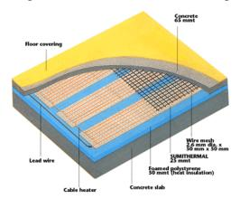
Figure 7.9 – Example of an electric floor heating system coupled with of PCM.
