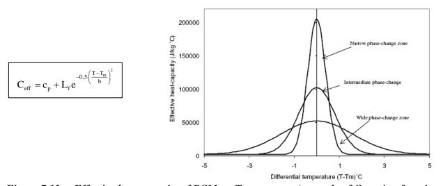
Figure 7.13 – Effective heat capacity of PCM vs. Temperature (example of Gaussian functions).
