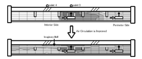
Figure 5.36 - Temperature distribution in the plenum during heat storage hours (top: without improvement, bottom: with the improvement).
