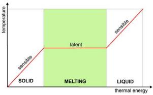
Figure 7.1 – Specific thermal energy (stored) vs. temperature.
