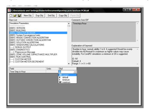
Figure 7A.2 – Example of the EnergyPlus menus –Time step selection.
