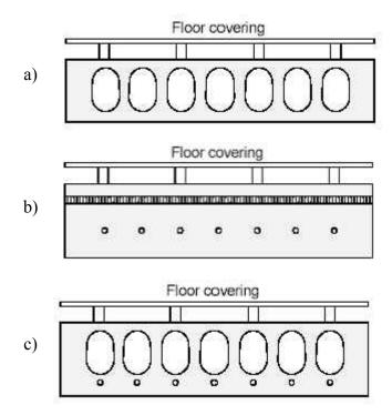
Figure 5.5 - Basic types of currently used thermo active building components (Wietzmann 2002): a) hollow deck with cavities for air circulation; b) on-site constructed floor (with insulation); c) hollow deck with integrated pipes (hollow can be also filled up with polystyrene or other light materials).
