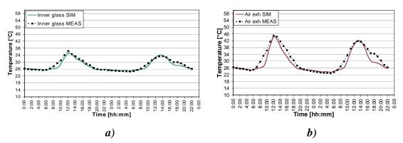
Figure 4A.1 – Simulated (continuous lines) and measured (symbols) glass (a) and air (b) temperatures, venetian blind configuration.
