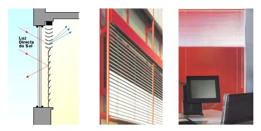
Figure 4.22 – Reflective double blade slope Venetian blinds.
