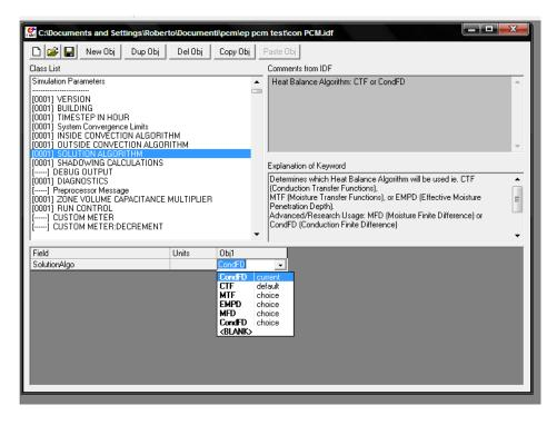
Figure 7A.1 – Example of the EnergyPlus menus – Solution algorithm selection.
