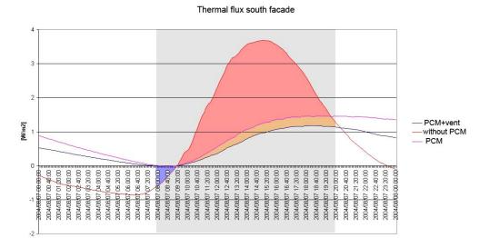
Figure 7.4 – Example of PCM application in walls – Specific heat flux through different type of façades (with - pink curve - and without - red curve - PCM; with - blue curve - and without - pink curve - ventilated cavity).
