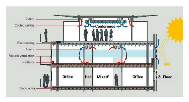
Figure 5.43 - Office building in Munich, installation of activated thermal mass components [Olesen (2000)].
