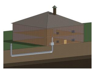
Figure 6.1 - Building with an Earth-to-Air Heat Exchanger.
