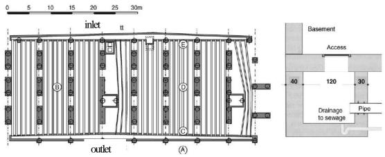
Figure 6.10 - General layout and construction detail of the ETAHE system in Schwerzenbacherhof building [Hollmuller (2002)].
