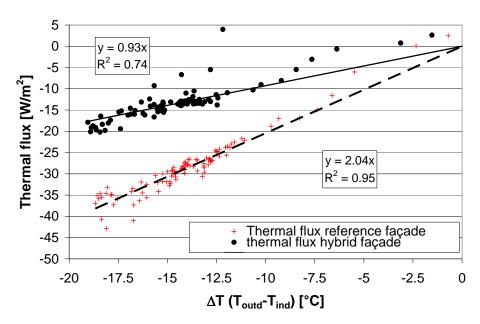
Figure 4C.2 – Transmittance of hybrid and reference façade, night time conditions.
