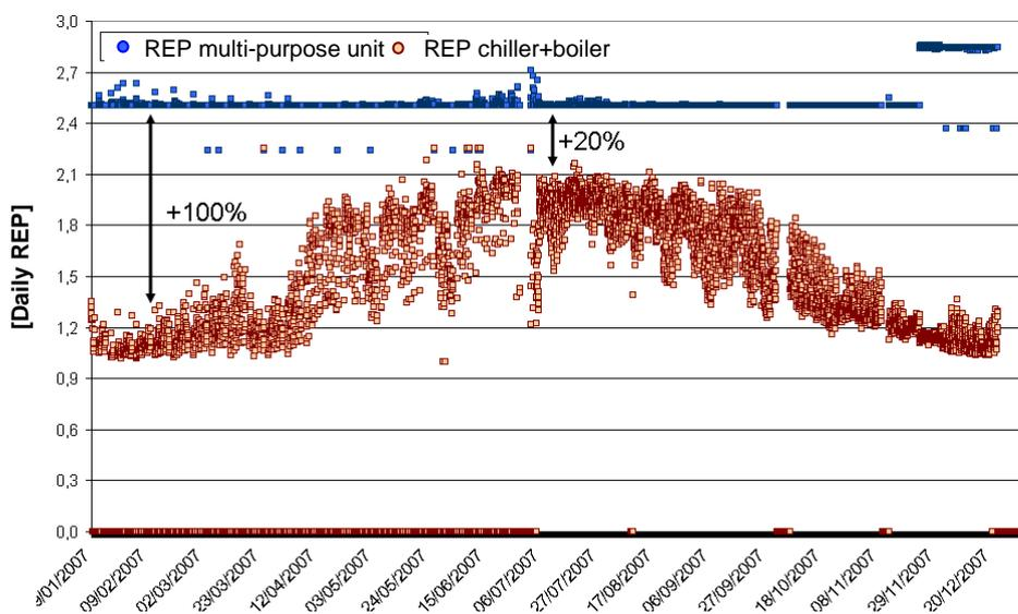
REP for the multi-purpose solution and for the chiller+boiler solution
