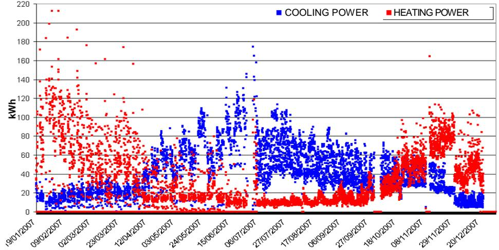
Heating and cooling energy given during 2007(hourly sampling rate)
