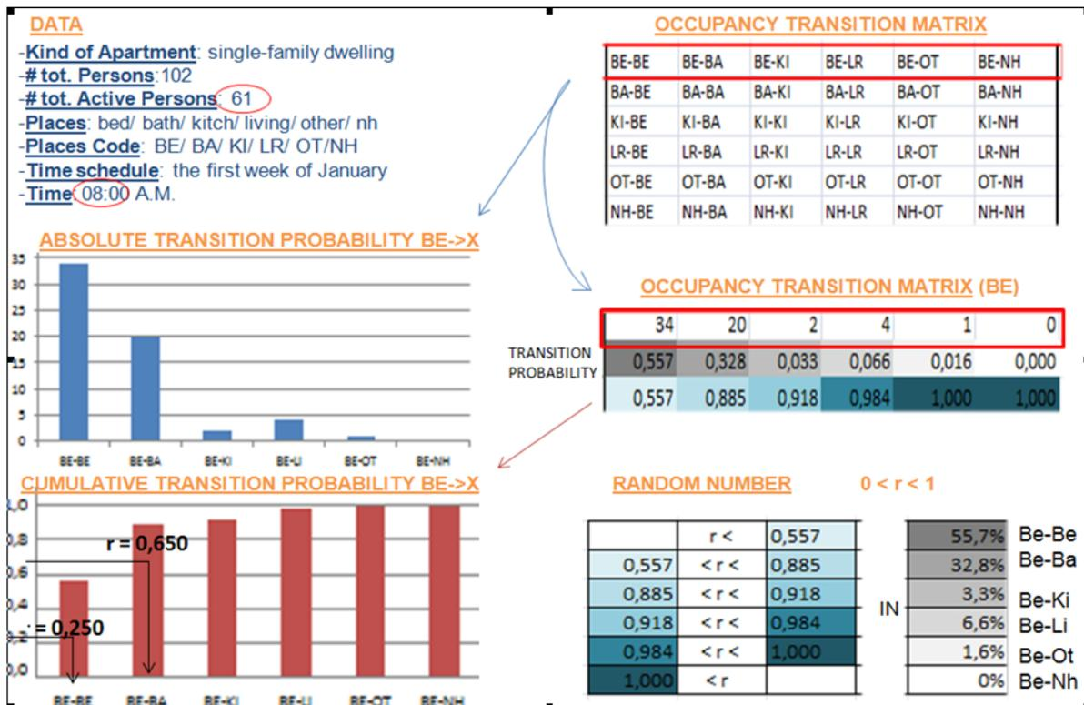
Figure 2-30: Schematic view of the Markov Chain Monte Carlo method for stochastically generating occupancy.
