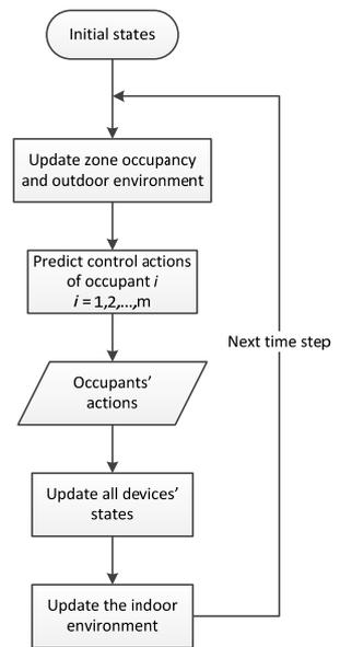
Figure 2-25. Workflow of control action models
