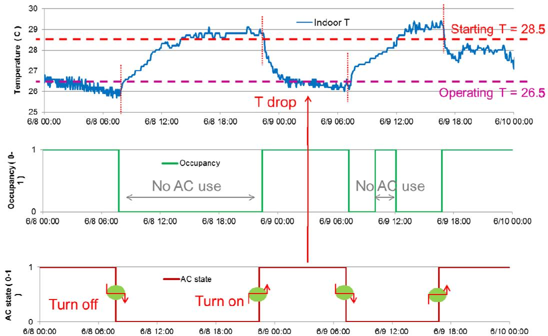
Figure 2-39. Simulation of air-conditioning behavior.
