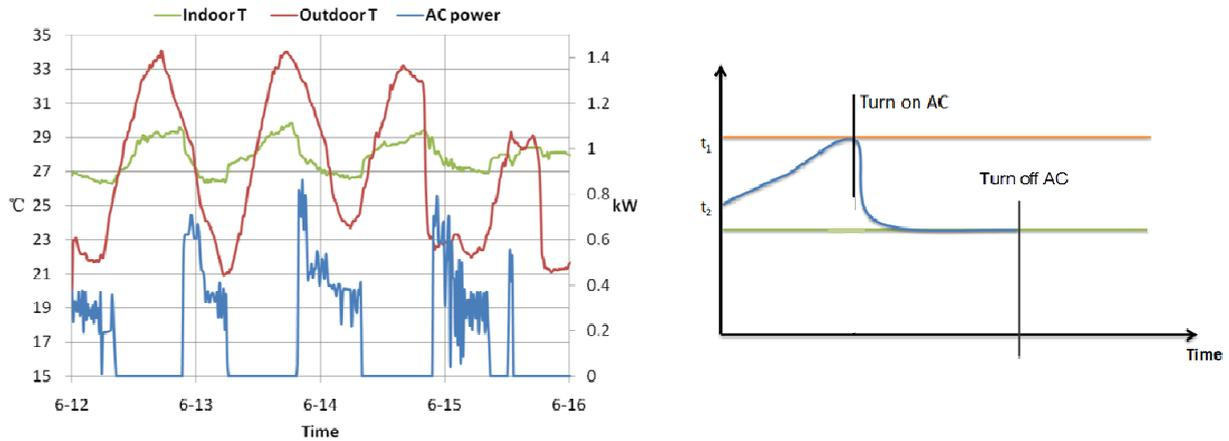
Figure 2-38. Air conditioner operation: (a) indoor and outdoor temperature, and AC power; (b) turn-on and turn-off patterns
