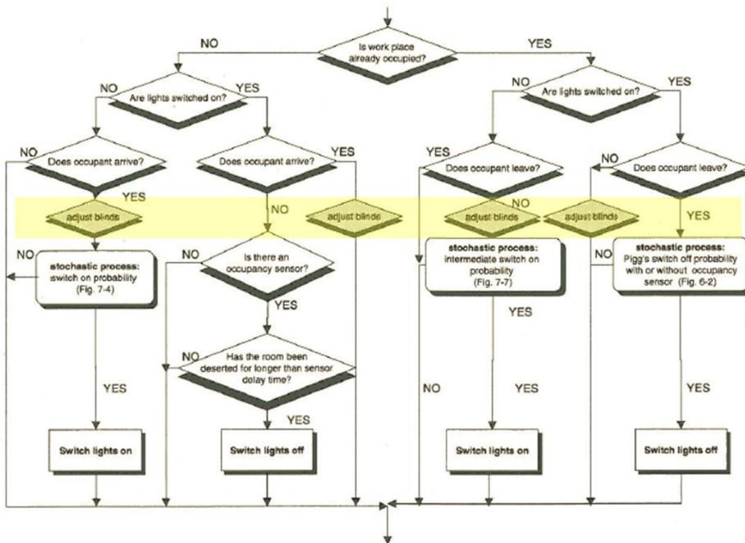
Fig. 8-6: integrated manual lighting control algorithm for blinds and artificial lighting.
