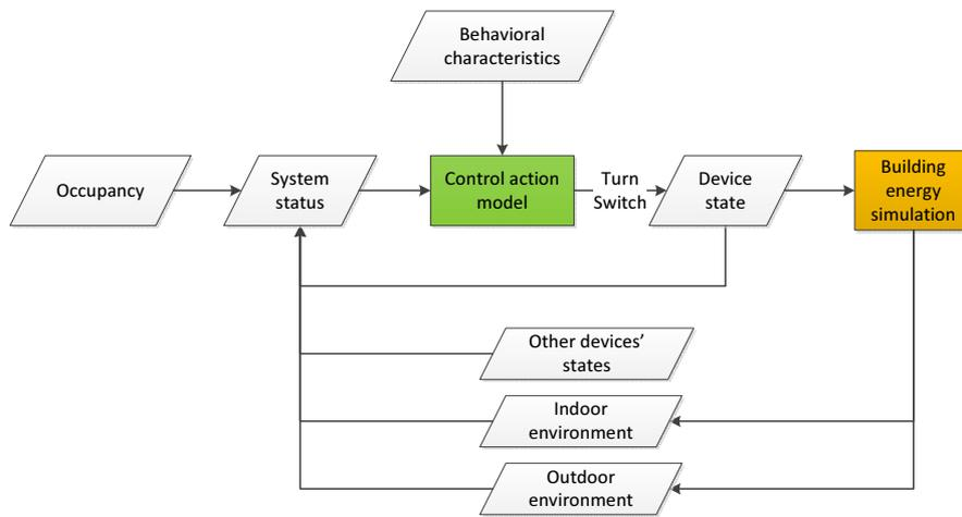
Figure 2-24. Schematic of each control action
