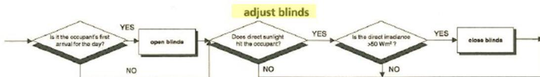
The control algorithms for manual blind control which are implemented in Fig. 8-6.
