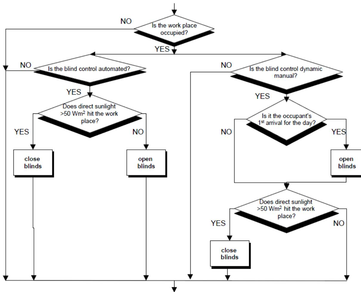
Figure 2-50: Control algorithms for manually controlled and automated blinds. Close blinds comes along with fully lowered blinds; the smallest slat angles are 0o, 45o and 75o is chosen under which direct sunlight is fully blocked, [70], p. 28].
