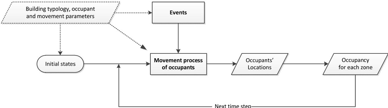
Figure 2-22. Schematic of the movement model
