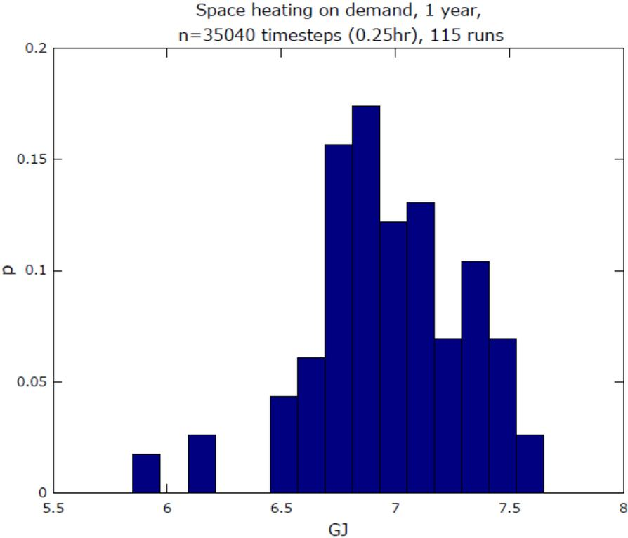
*Figure 2-32: Histogram of the yearly energy use for on-demand space heating for a two working person household following from the alternative Monte Carlo procedure based on sampling the above described deterministic occupancy profiles.*
