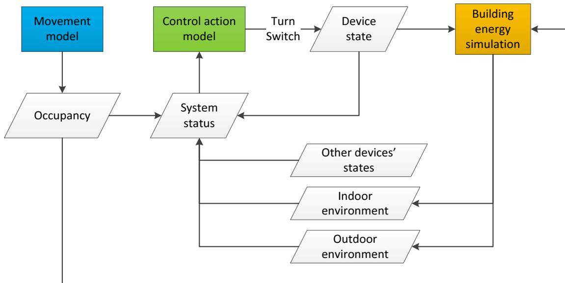
Figure 2-26. Integral workflow of occupant behavior model and existing building simulation tool.
