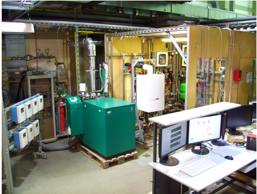
Figure 2. Test facilities for micro-cogeneration systems.
